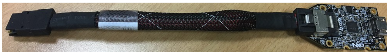
Figure 2. i.MX mini SAS cable with LVDS-to-HDMI adapter
